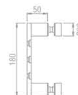
DS1S S.S. Side Bracket to Hold Glass
